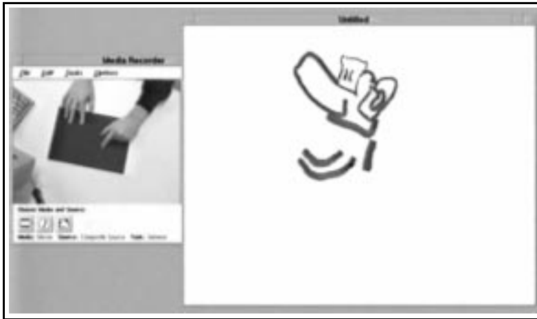
Fig. 9. The drawing package in action. This screen shot shows a cartoon character drawn using the drawing package; note the variable-width lines. A movie clip showing this figure being created is available at [15]. The scene on the left is the camera's view; it is shown for information only and is not employed by the user.
