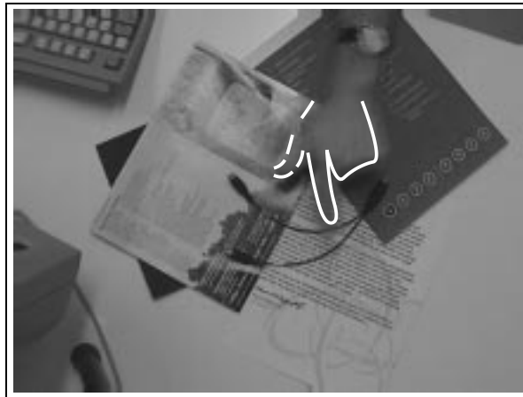
Fig. 4. Heavy clutter does not hinder the hand tracker. Even moving the papers on the desk to invalidate the background subtraction does not prevent the Condensation tracker functioning. The fingertip localisation is less robust, however, and jitter increases in heavily cluttered areas.
