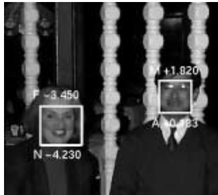
Figure 1. Two detected faces and the associated gender (Male/Female) and ethnicity (Asian/Non-asian) estimates. Following the label is the classification confidence.
