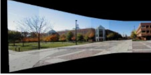
Figure 4. Image alignment using the refined homography estimates.
