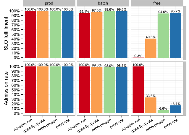
Figure 3. Percentage of requests with VM availability SLOs fulfilled (top graphs) and admitted (bottom graphs) per class in the base scenario.
