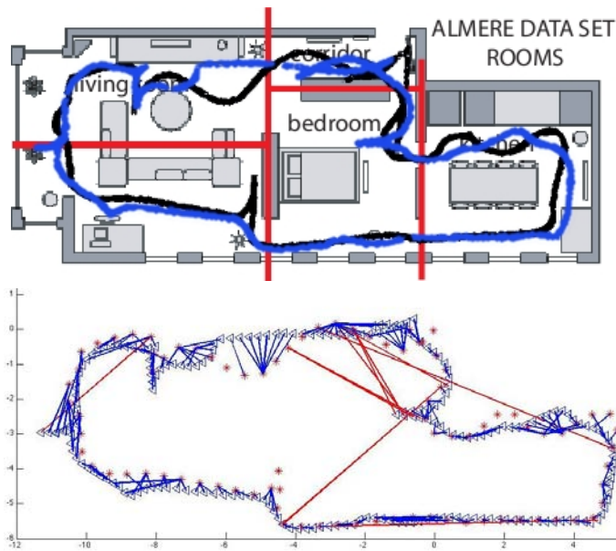
Fig. 9. Experiment 3. Localization with indoors dataset. Top image shows the environment scheme and the room-clustering (red lines are cluster limits) and the odometry from runs 1(black) and 5 (blue). Bottom image shows the localization results summary with the E_{omni} (0) approach.
