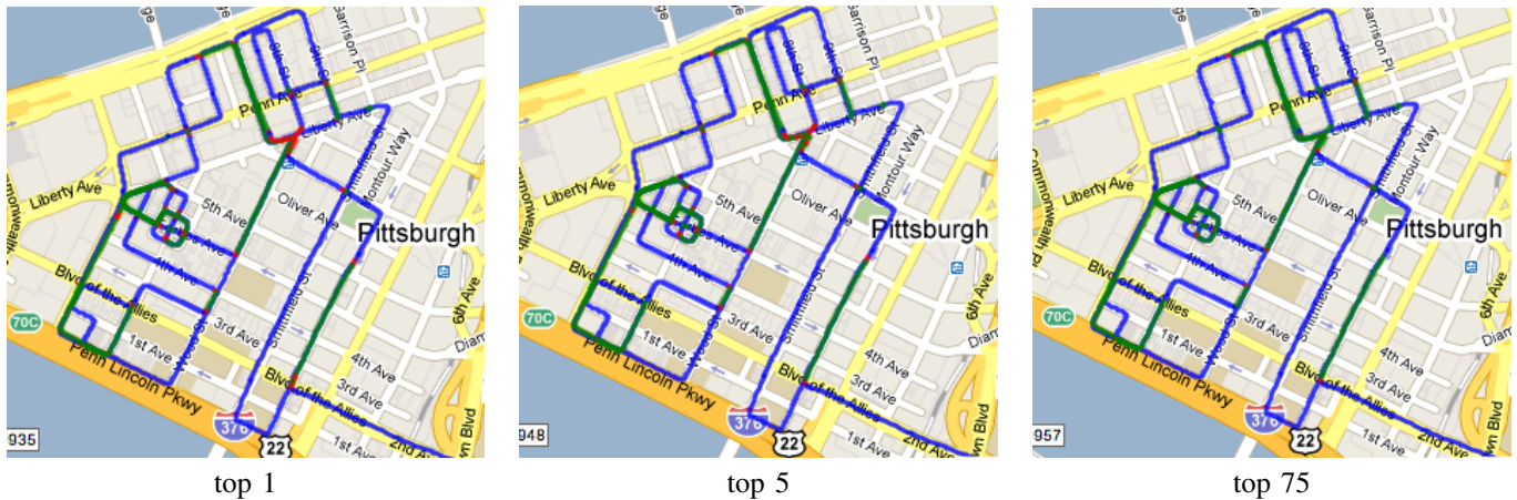
Fig. 5. Visualization of correct loop closures and their associated accuracy. Green line are the correctly identified locations, red line are the locations of false negatives which our method missed. The above graph plots the results evaluating whether the closest reference view among top k nearest views to the query view.
