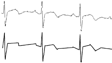
Figure 51.13. An example of a time series segmentation with its piecewise linear representation
