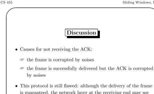
• This protocol is still flawed: although the delivery of the frame is guaranteed, the network layer at the receiving end may see multiple copies of the frame.
