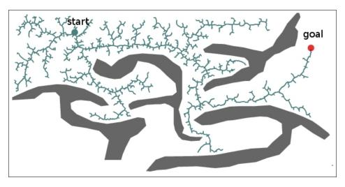
Figure 6: The tree built by RRT is shown here on a simplistic environment.
