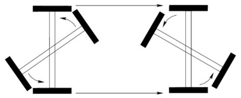
Point wheels as in destination. Translate. Rotate to desired orientation.
