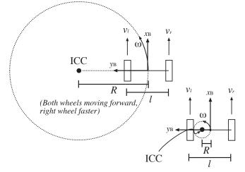
*(left wheel moving backwards, right wheel forward and faster)*
