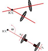
For ddrive, ICC exists as long as  $v_{\ell} \neq v_r$ . Ddrive rotates around ICC.
