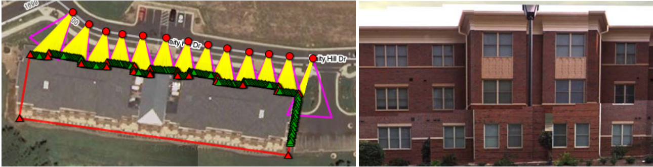
Figure 9. The left image shows the views selected for the top portion of a building from the Baity Hill dataset (the views selected for the bottom part look very similar). The right images shows a view generated with the synthesized 3D model.
