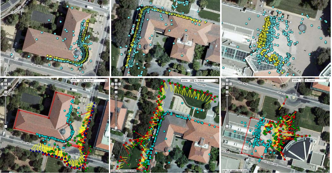
Figure 3. The top row shows alignment of the 3D reconstruction points projected on the ground plane after the initial RANSAC alignment (cyan) and after final ICP alignment (yellow). In addition to good alignment, all the outlier points have been removed. The bottom row shows the camera poses (green dots are original GPS readings connected by a line to the corresponding red dots indicating computed camera locations; yellow lines indicate viewing directions) and the aligned reconstruction points. The red contours show building outlines.
