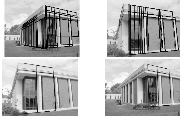
Fig. 10. Library image pair: structure detected in the first view (upper left); structure detected in the second view (upper right); successfully matched structures (bottom).
