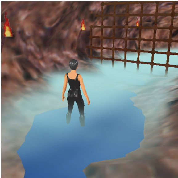
Figure 10: Mystic Cave - Heterogeneous Fog based on Perlin noise functions in 2 dimensions, and a height based exponential function
